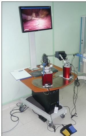
Figure 1: LapSIM® virtual reality simulator (Surgical Science AB) with haptic feedback Xitact™ IHP, Mentice AB, Sweden. IHP: Instrument haptic ports
