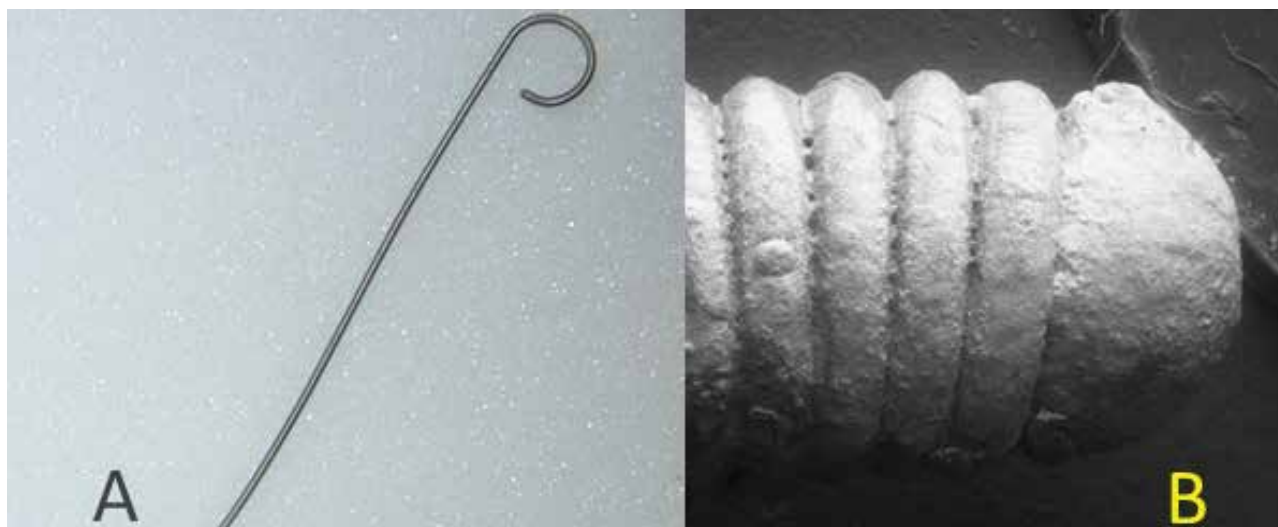
Figure 1A: An Resonance stent after 12 months of indwelling. Notice that encrustation is not evident on the stent
